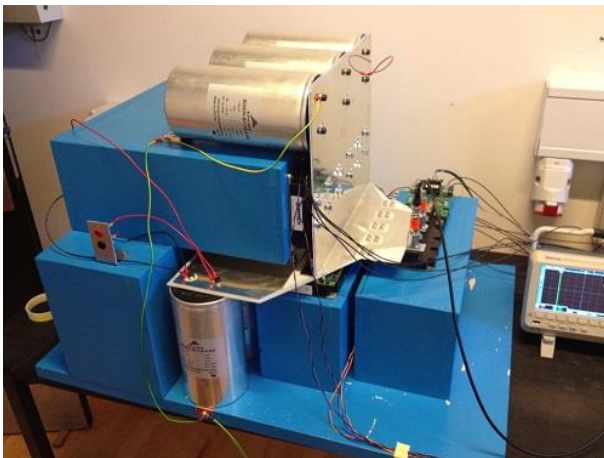
(c) A non-destructive short circuit testing system for high-power IGBT modules (up to 6-kA current level.)
