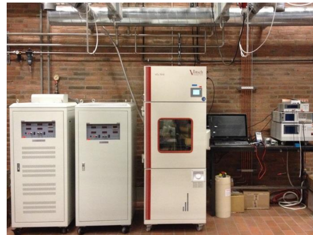
(d) A capacitor testing system (up to 2-kV voltage and 100-A ripple current under climatic conditions).
