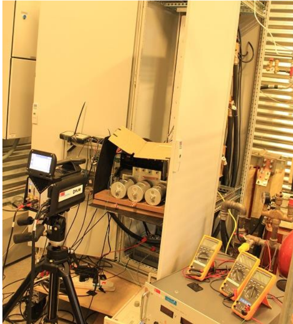
(e) A power cycling testing setup under open module test with infrared camera for direct junction temperature measurement.
