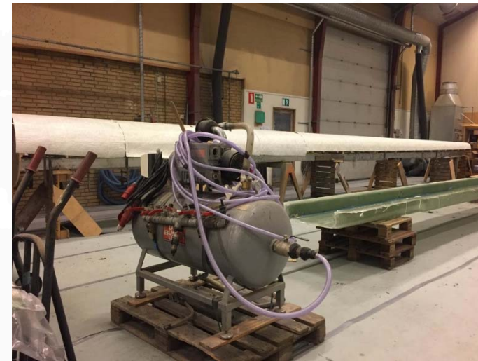
Fiberglass / epoxy rod made by 'hose' method
