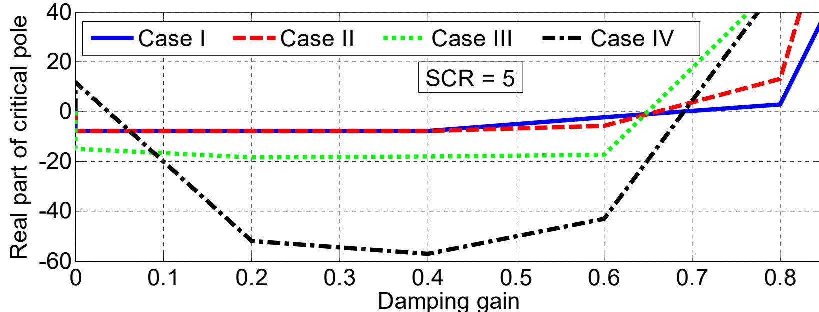
Real part of the critical pole in terms of damping controller gain ( $K_d$ ) for different cases under SCR = 5.
