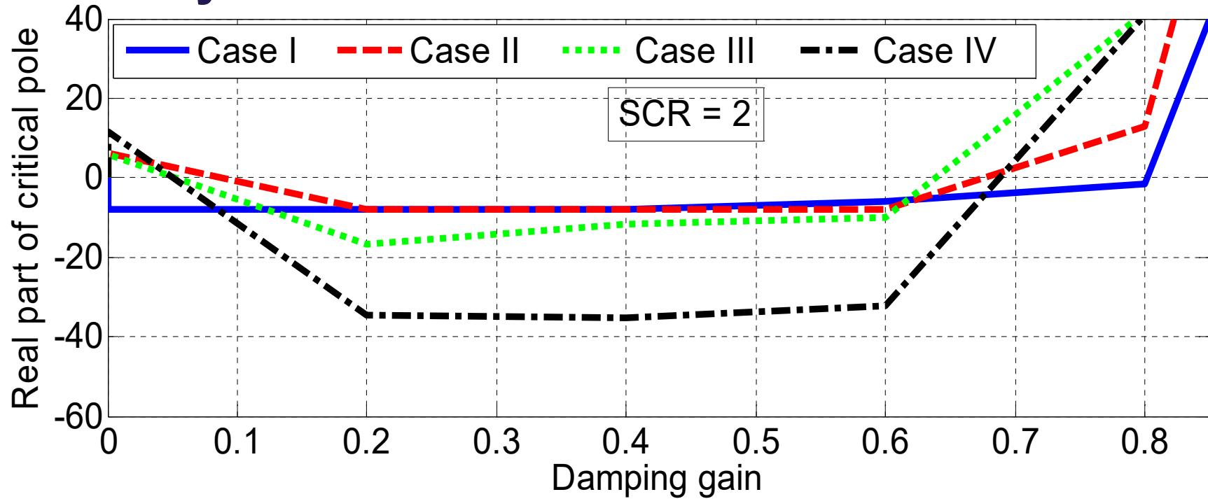
Real part of the critical pole in terms of damping controller gain ( $K_d$ ) for different cases under SCR = 2.
