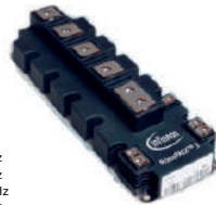
1700V, 1000A IGBT module under test
