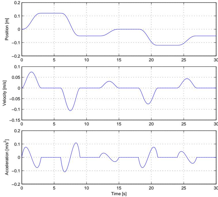
Figure 5: Plot of the input reference trajectory for the cylinder position.
