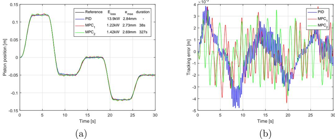
Figure 9: Comparison of position tracking results the developed controllers.
