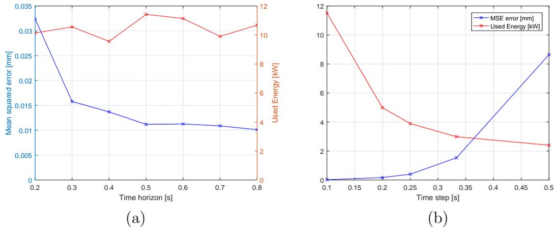
Figure 6: Energy and mean squared error for various time step and horizon length.
