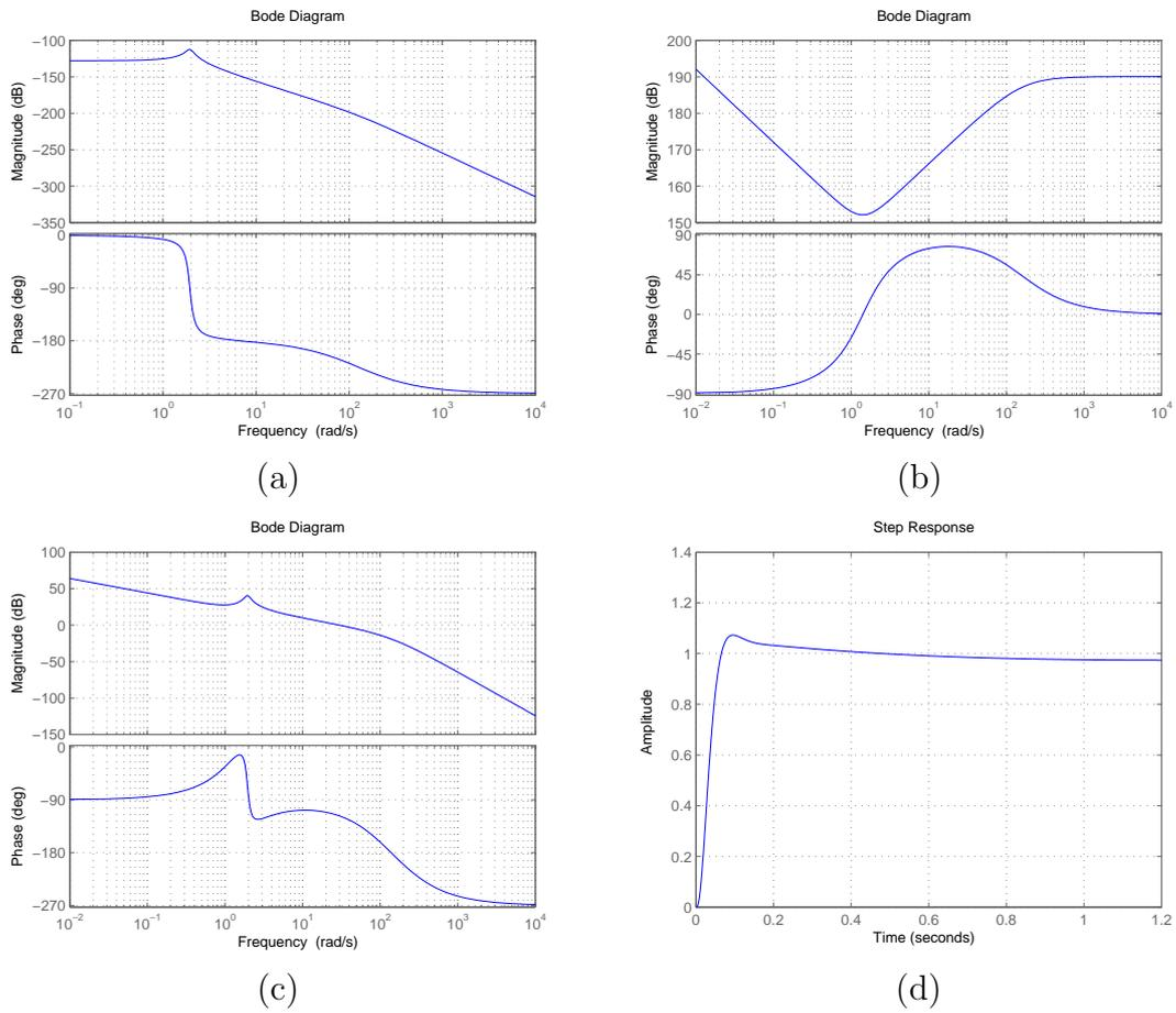
Figure 4: (a) Uncontrolled system with force dynamic approximations. (b) The applied controller. (c) Controlled open loop system. (d) Closed loop step response.
