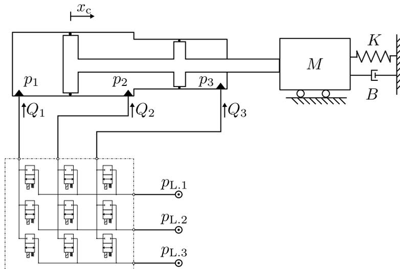
Figure 1: DDC force system and the load system.
