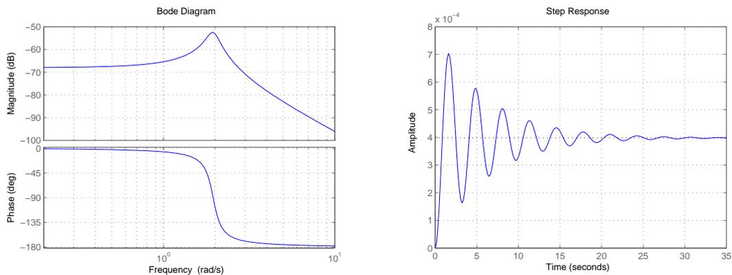
Figure 3: Bode diagram and step response of the load system,  $G_p(s)$ .
