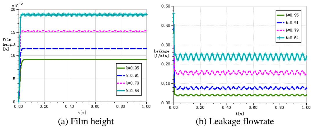
Figure 8. Film properties in different pressure ratio  $b$
