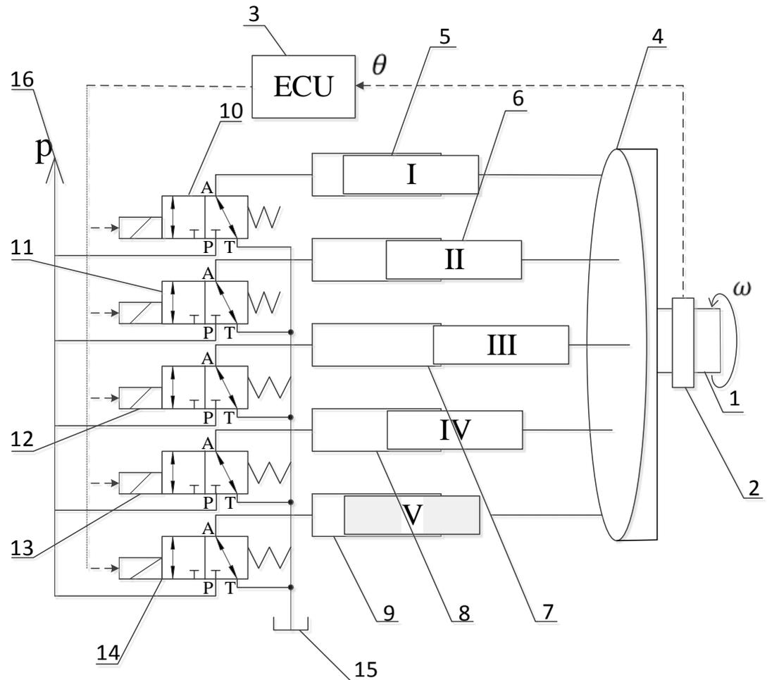
Figure 1. Schematic of the axial piston pump with digital distribution
