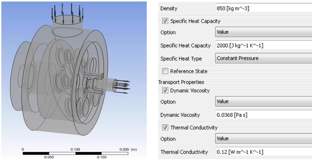
Figure 9. Heat transfer simulation domain and its settings
