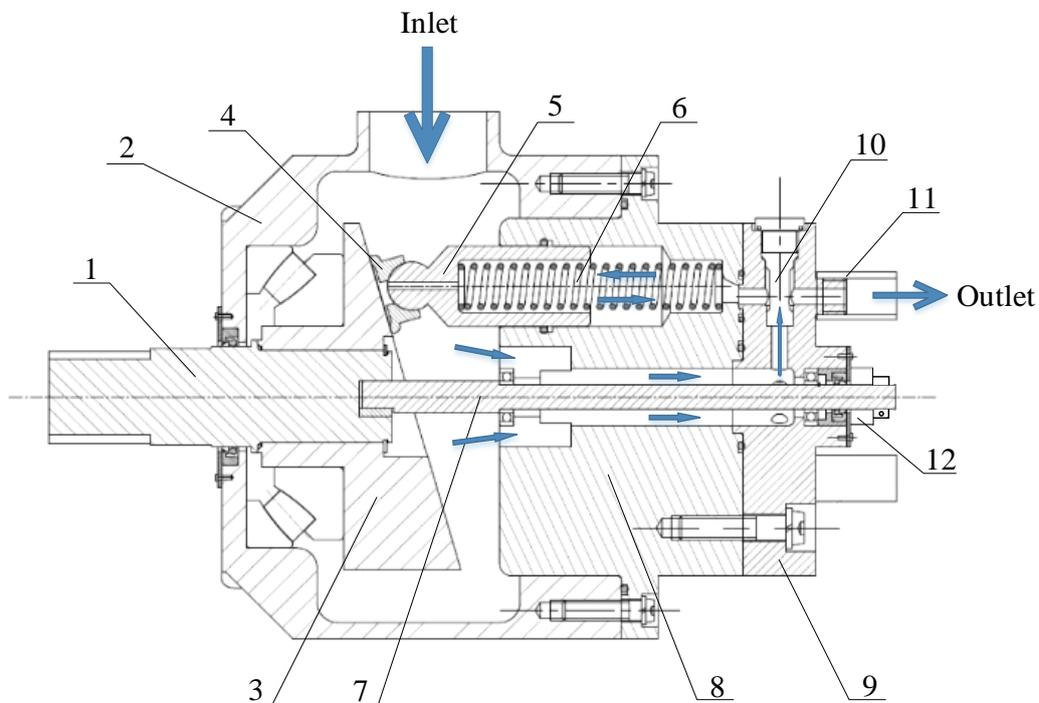
Figure 2. Structure diagram of the new axial piston pump with digital distribution (1.Input shaft, 2.Low-pressure body, 3.Swash plate, 4.Swash shoe, 5.Piston, 6.Spring, 7.Secondary shaft, 8.Barrel, 9.HSV body, 10.2/2 way HSV, 11.Check valve, 12.Absolute encoder.)
