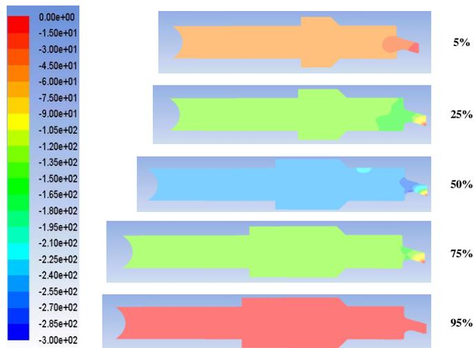
Figure 6. Pressure distributions in piston chambers at different time
