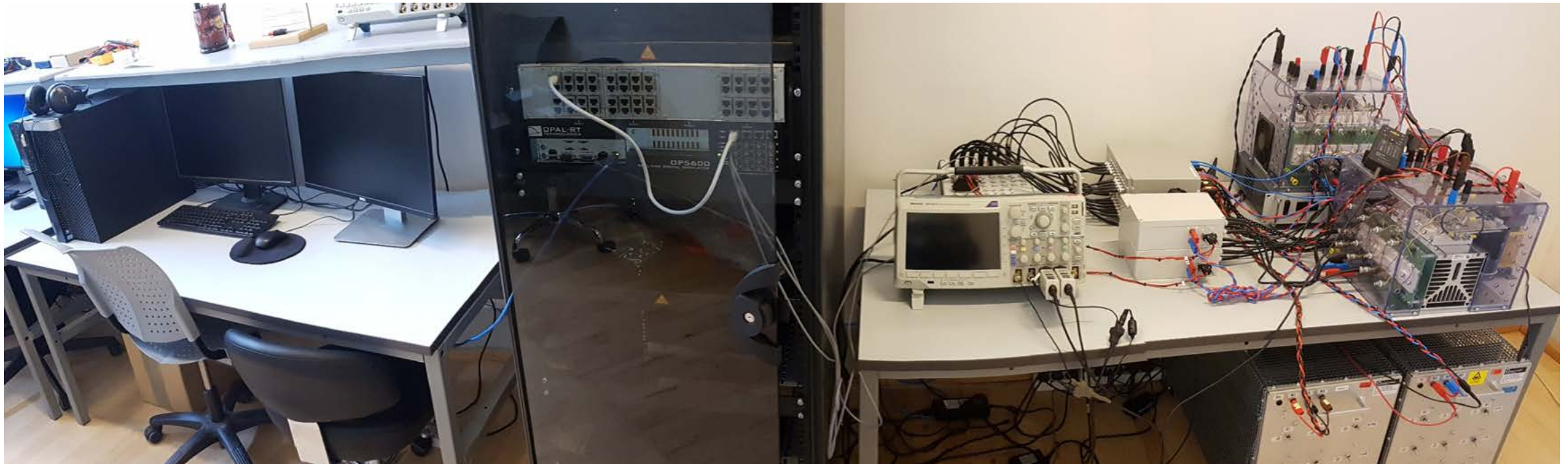
Fig. 3. Power hardware in the loop experimental setup.
